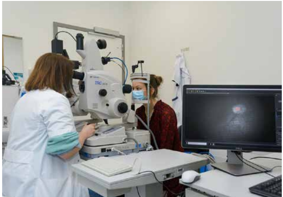
Set-up of combined hyperspectral and fundus camera at Peter Stalmans’ lab at KU Leuven
