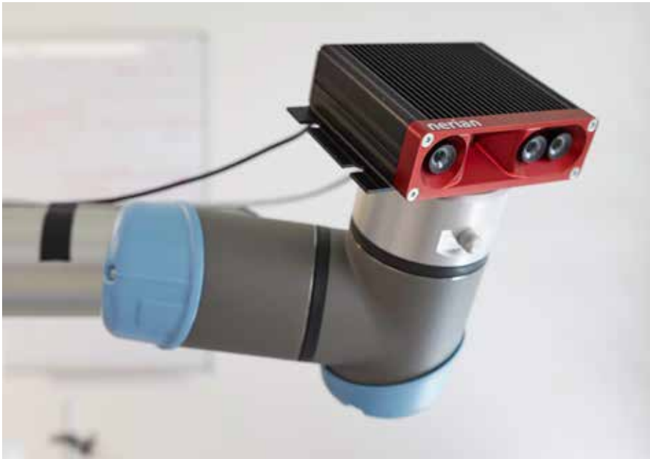
Nerian Vision's stereo vision cameras incorporate an FPGA for real-time 3D imaging
