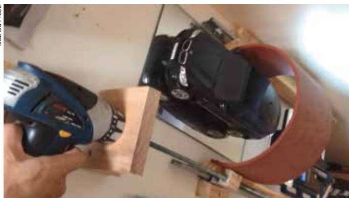
Isak du Preez's first prototype scanner, built in 2016 from hardware store materials
