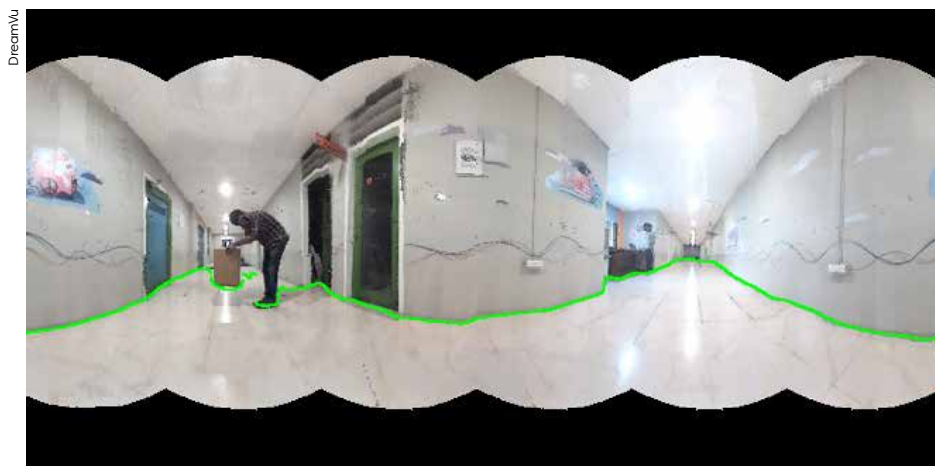
The PAL omnidirectional image sensor from DreamVu has a series of curved surfaces that capture light from all directions at multiple points on the sensor. This is converted into two RGB panoramic images from which distances can be calculated
