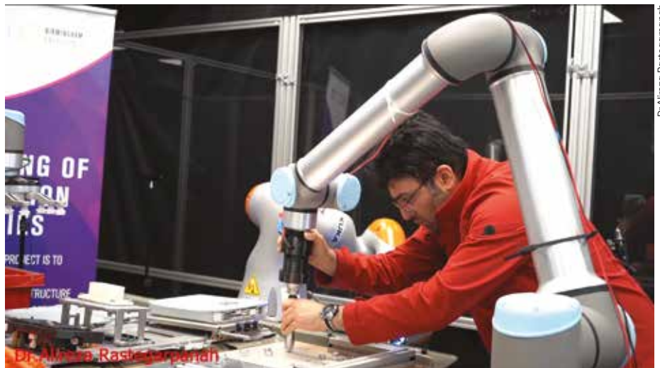
Dr Alireza Rastegarpanah working with a cobot on the task of unbolting a lithium-ion battery.
