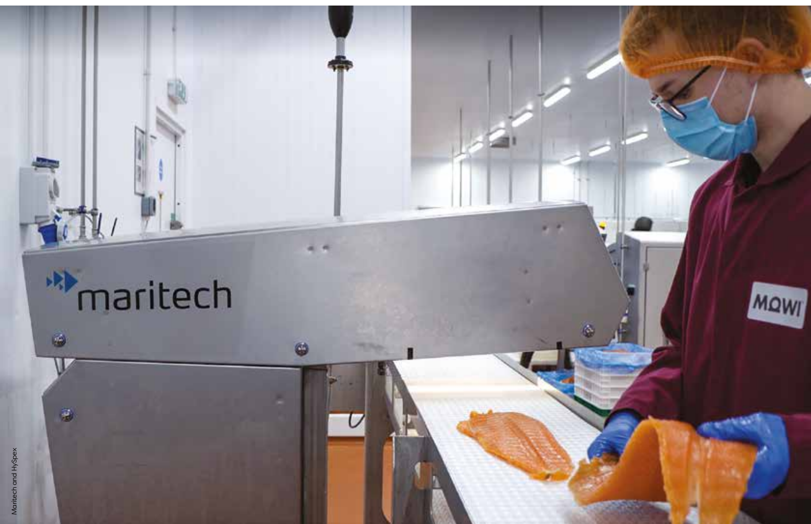
The Maritech Eye system uses hyperspectral imaging to gauge the quality of filleted fish
