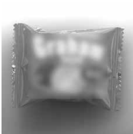
Shortwave infrared imaging can be used to image products through plastic packaging, as well as check for fill levels in bottles
