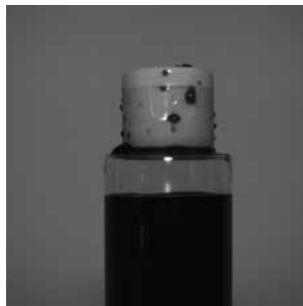
Shortwave infrared imaging can be used to image products through plastic packaging, as well as check for fill levels in bottles
