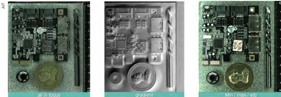
Enhanced, rectified 2D images produced by inline computational imaging
