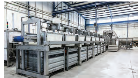
Each tuna is automatically sorted into its appropriate container
