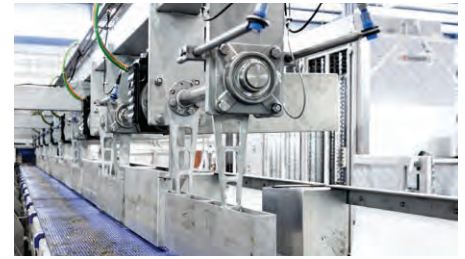
Tuna are scanned by two Matrox Altiz before being classified; 3D classification results and location data is sent to the sorting section
