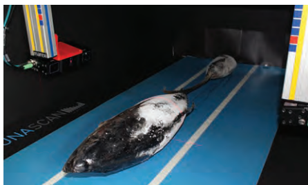
Two Matrox Altiz 3D profile sensors (on the far left and right) scan each fish as it passes through the dual-sensor TUNASCAN system
