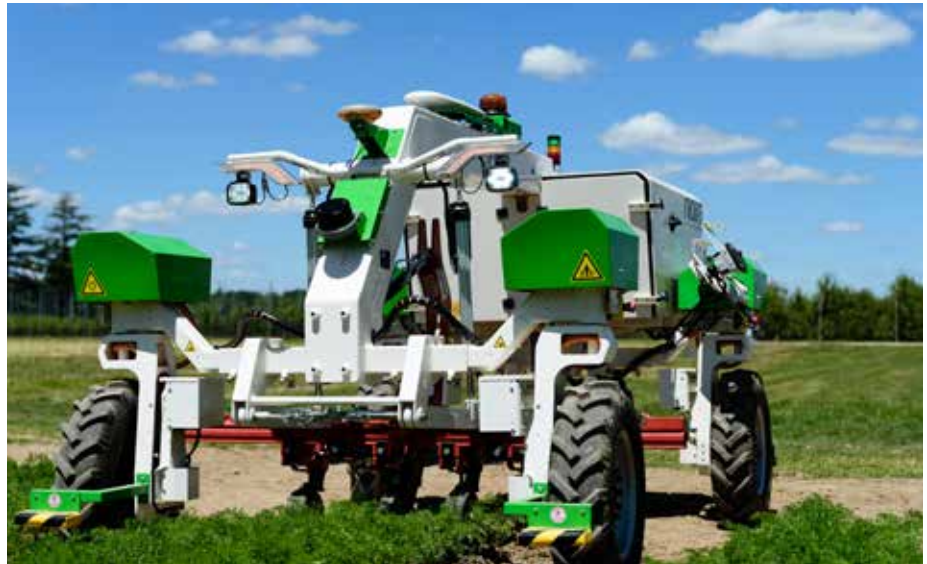
Naïo Technologies' tool-carrying Orio robot uses lidar to increase safety levels and work faster
