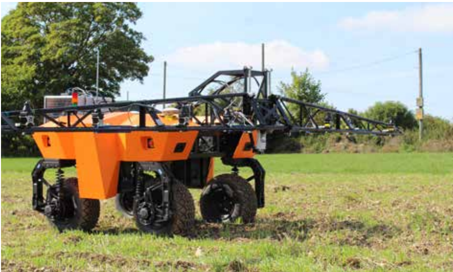
SRC's Tom V4 uses eight 6MP cameras to monitor a field, down to individual water droplets on leaves
