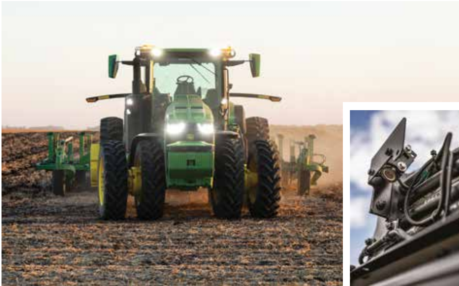
John Deere's 8RX feeds two NVIDIA GPUs from six pairs of cameras, inset, for obstacle detection
