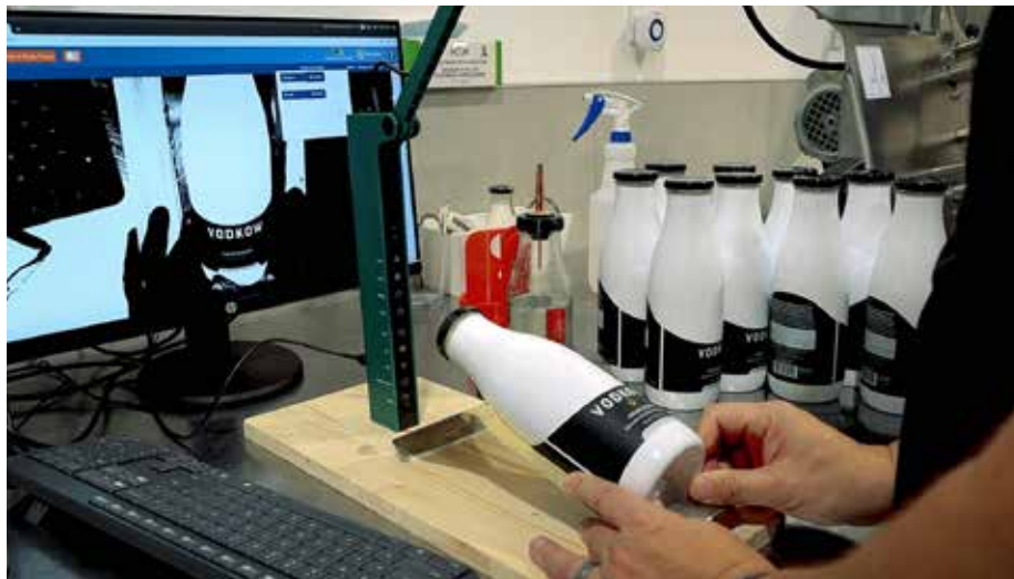
Trialling visual inspection tools at a distillery, as both a visual learning tool for new employees so they can learn required brand elements, and as a pass/fail QC check to verify all elements are on a bottle
