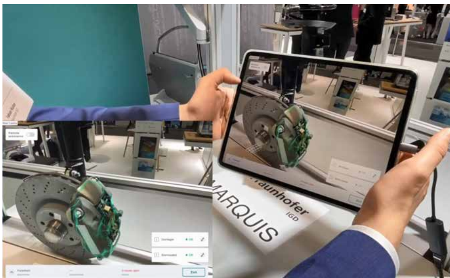
Top: Is the component in the correct position? If not, the AI-based MARQUIS software superimposes the relevant element in red. Above: Using augmented reality, the inspection engineer is able to see on the tablet that the structure is free of defects. The component is now overlaid in green.
