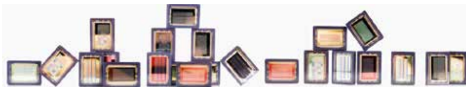
Imec hyperspectral sensors, with spectral filters deposited directly on top of image sensors
