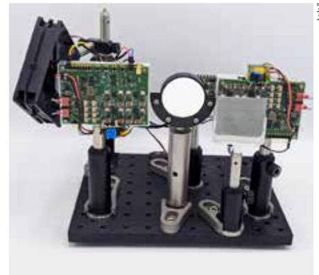
The 1,130nm SWIR 3D camera is a good fit for outdoor sensing applications
