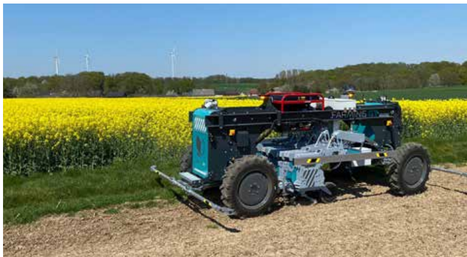
Above and right: Farming Revolution’s Farming GT robot uses a multispectral camera to take high-res images of plants. A deep neural net identifies weeds before a rotating chopper cuts them off at the stem
