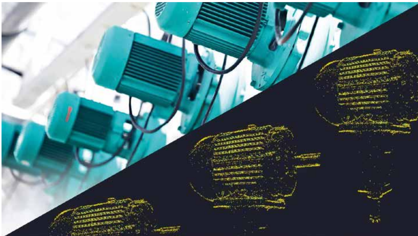
Event vision can trace particles or monitor vibrations with low latency, low energy consumption, and relatively low amounts of data
