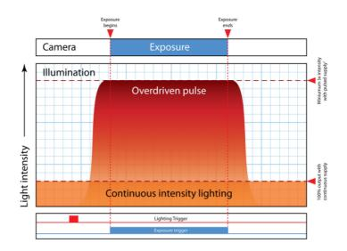
Overdriving is used with pulse lighting and it brings benefit to most Vision applications. The exceptions are applications where the camera is exposed for a high percentage of the time, for example Line Scan applications.
