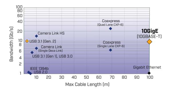
The next generation of high-performance CMOS sensors will open the door to exciting new vision applications, but taking advantage of them will depend on whether your interface can keep up. Ethernet and USB interfaces are increasing their transfer rates to 10Gb/s, adding to the strengths that make them dominant camera interfaces. What are these new technologies and are they ready for machine vision use?
