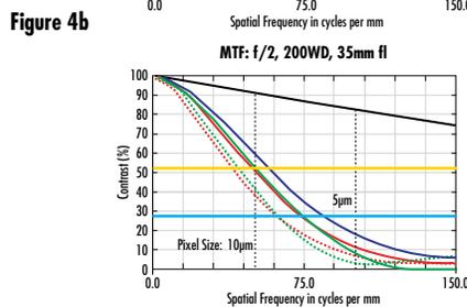
Figure 4: MTF curves for a 35 mm lens at the same WD and different f/#s: f/4 (a) and f/2 (b)
