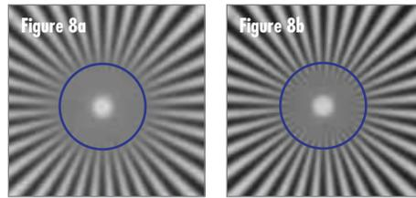
Figure 8: Images of a star target taken with the same lens, at the same f/#, with the same sensor. The wavelength is varied from 660 nm (a) to 470 nm (b)
