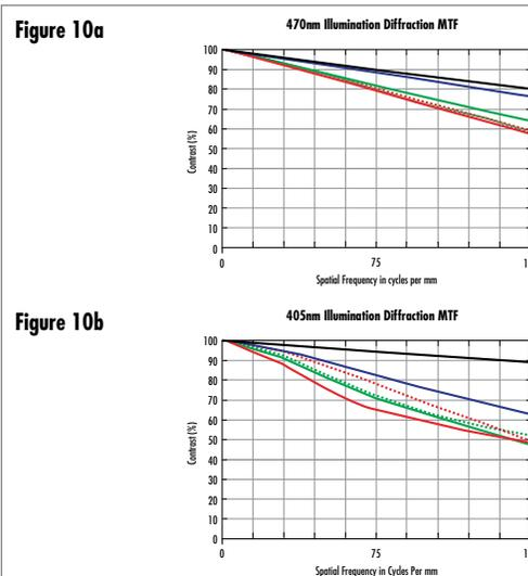
Figure 10: MTF curves for a 35 mm lens at f/2 with 470 nm (a) and 405 nm (b) wavelength illumination
