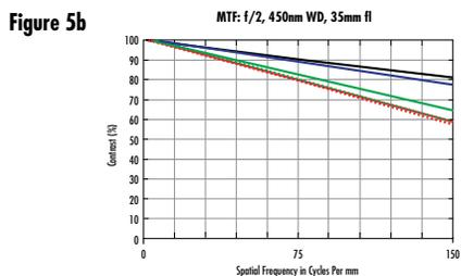
Figure 5: MTF curves for a 35 mm focal length lens at f/2 with different working distances
