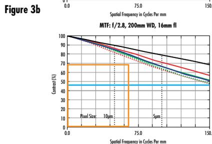
Figure 3: Two different high resolution lens designs with different focal lengths at the same f/# and system parameters
