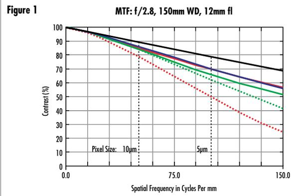
**Figure 1:** MTF curve for a 12 mm lens used on the Sony IXC 625 sensor
