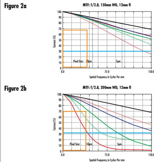
**Figure 2:** MTF curves for two lens designs (a and b) with the same focal length,  $f/\#$ , and system parameters
