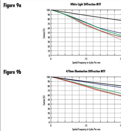
Figure 9: MTF curves for the same lens at f/2 using a different wavelengths; white light (a) and 470 nm (b)
