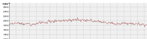
Pixel response before gain and offset correction
