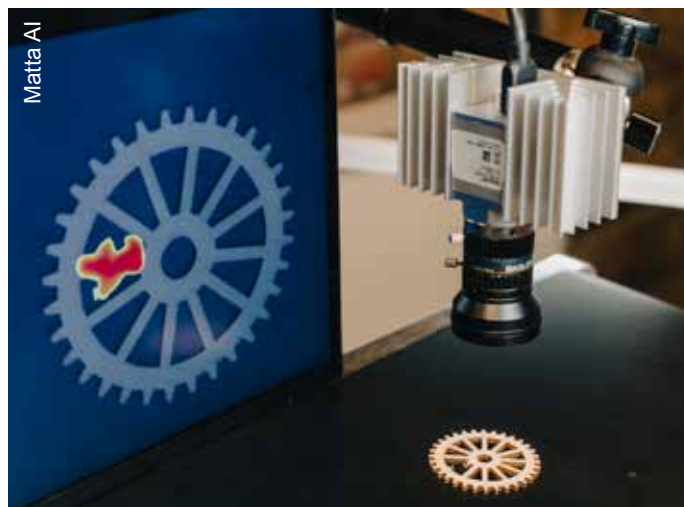
Matta's AI vision-based quality control system detects defects as part of the manufacturing process
