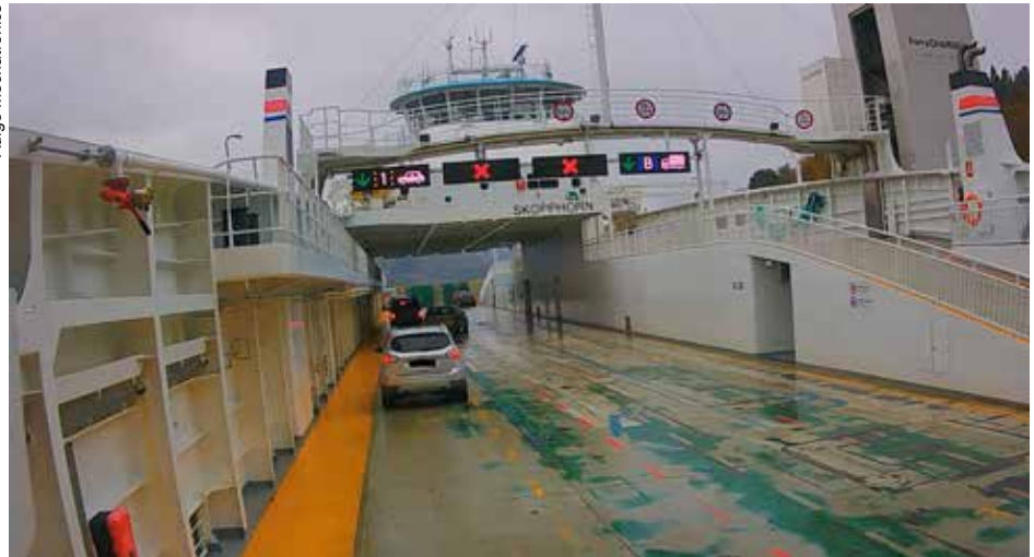
The automated RoRo vehicle guiding system uses computer vision-controlled signage to direct drivers onto the ferry
