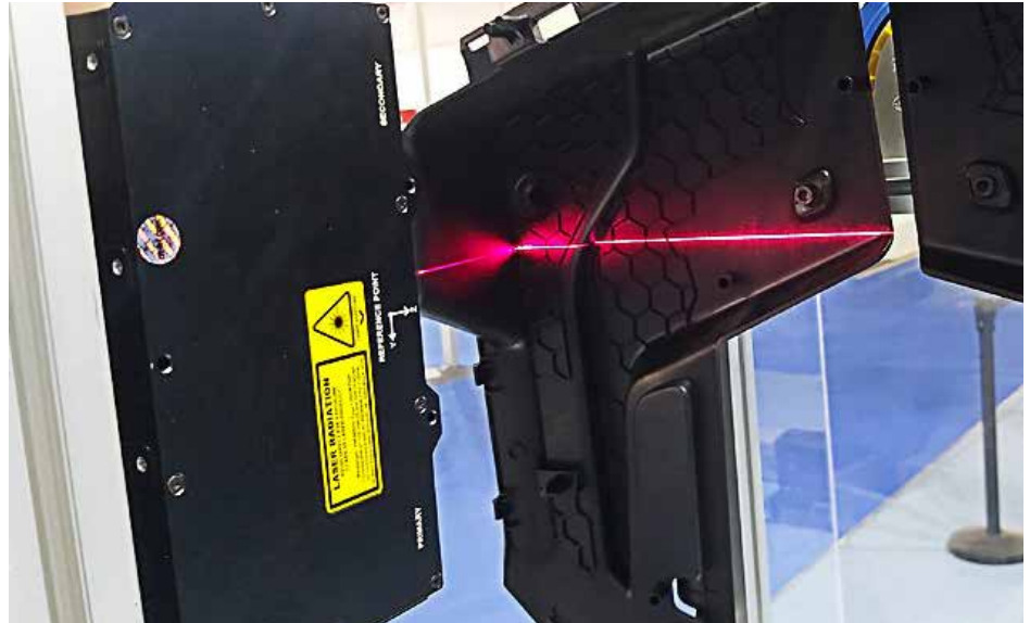
Sentinel's 3D laser inspection system to detect defects on plastic injection-moulded parts for the automotive industry was "especially complex", said Oliveira
