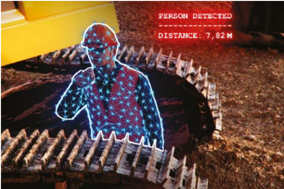
The Visionary AI-Assist system detects people and objects in dangerous positions near to moving vehicles
