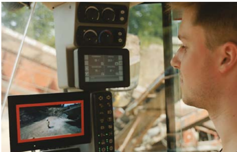
How the AI-based system assists users by detecting people and objects
