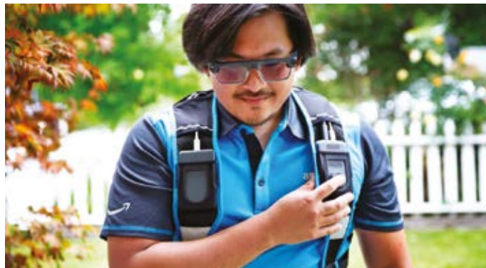
The system is completed by a vest that includes operational controls, a swappable battery and an emergency button
