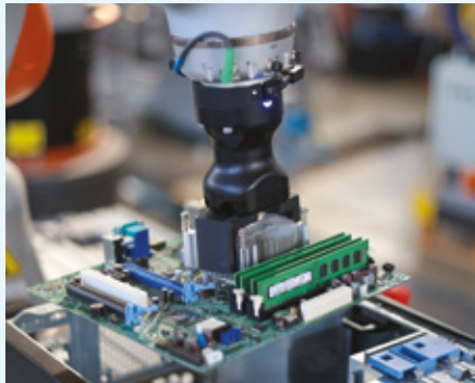
Robot lifts the motherboard out of the housing
