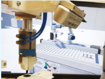
Guided by 3D data, the robot picks up a clip and inserts it into a moving part
