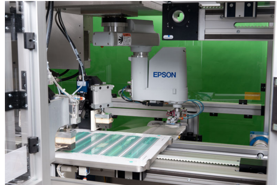
Two additional GigE cameras identify and locate the corresponding features on each lid. Sherlock vision software performs calculations and provides X, Y, and rotational correction values, which an Epson robot uses to position the lid on each coupon accordingly.
